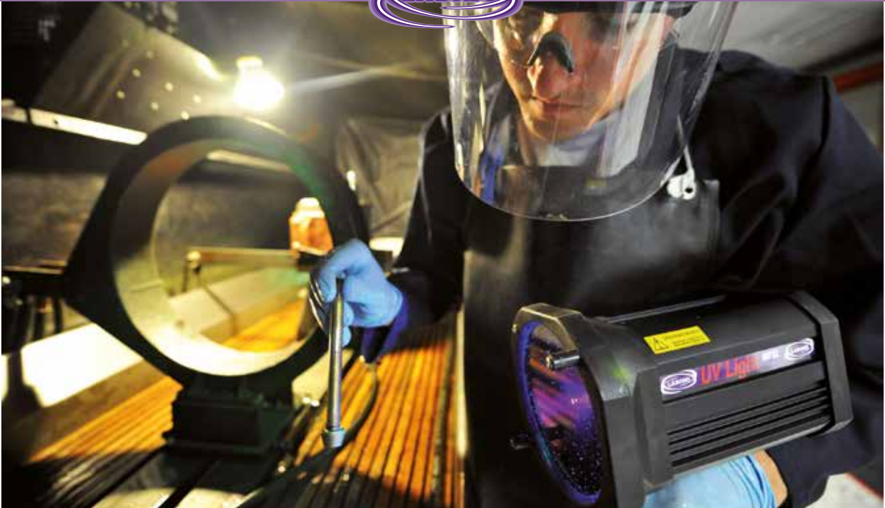
NDI Technician of the 86th Maintenance Squadron takes a closer look at a nose landing gear wheel bolt during a magnetic particle inspection at Ramstein Air Base, Germany.
