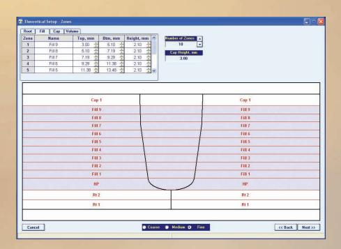
Ray Tracing screen for determining of zone-by-zone insonification scheme (pulse echo or tandem; incidence angles; emitting and receiving aperture; focal distance) and appropriate positions for phased array probes from both sides of the weld
