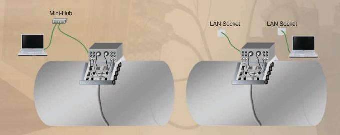
Thanks to innovative architecture there is no need in bulky long umbilical for probes connection. Each probe is plugged into appropriate socket of **ISONIC PA AUT Platform** using short cable – this significantly increases signal to noise ratio and simplifies placing / removal of scanner or tractor onto / from object under test and scanning as well
