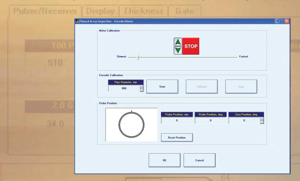
■ Each probe either phased array, conventional pulse echo, or TOFD may be driven independently through appropriate pulser receiver. This feature is very useful for various purposes such as verification of wedges, studying of phased array focusing effects, etc
