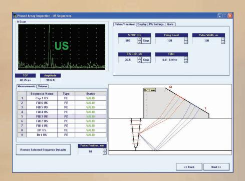
■ Conventional and TOFD Probes Channels Settings screen for calibration of firing pulse amplitude and duration, gain, etc according to inspection schemes to be implemented
