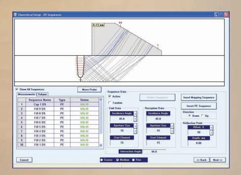
Theoretical Setup file is created upon completion of wizard as described and used for further setting of phased array channels
