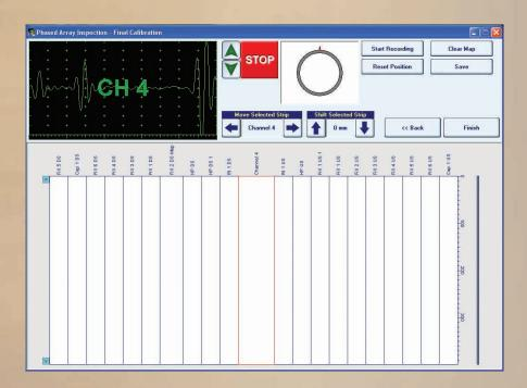
Ultrasonic Setup Wizard is finished with creation of complete Inspection Setup File; inspection becomes possible at any moment after said file is uploaded into scanning routine
